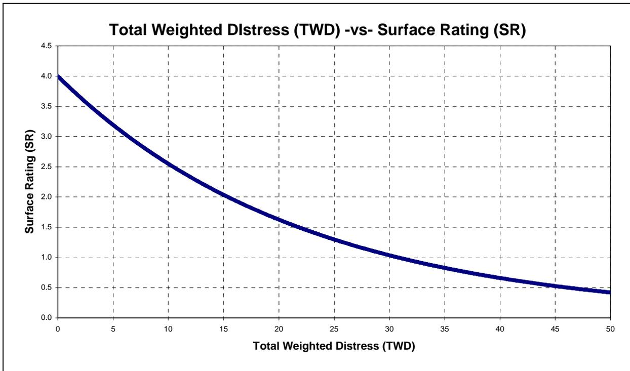
**Figure 7. Chart for Converting TWD to SR.**
