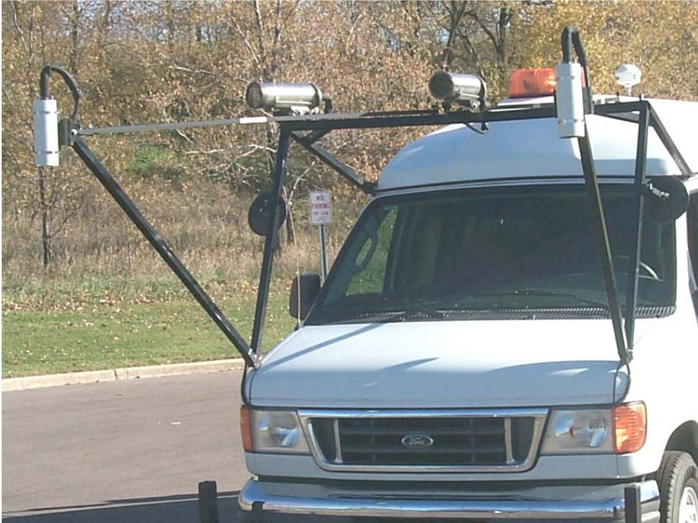
**Figure 4. Close-up of cameras used to record pavement distress.**
