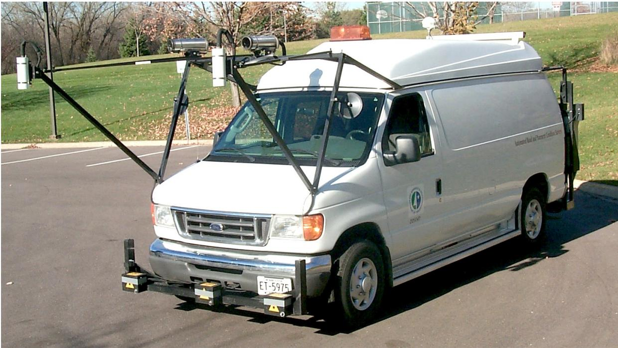
**Figure 1. Mn/DOT's Pathway Services, Inc. Digital Inspection Vehicle (DIV)**
